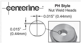
When facing the head, add a 0.015" (0.4 mm) counterbore, 0.015" (0.4 mm) deep (as shown). This will minimize arcing and binding of the pin in the event the part being welded has a sharp edge or burr around the hole.
